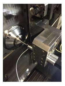
Possibility of centering "horn" or "gooseneck" devices in front of guide bush. Can also be used on the counter-spindle or directly on the fixed / revolving guide bushes.
