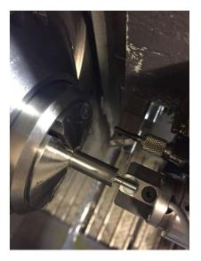
Each tool position on multiple supports can be centered without the need to disassemble the tools near the machining station. The setup of adjustable tool holders is greatly facilitated.
