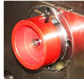
Then lay the probe holder bushing on the material bushing and secure it with the locking screw.
