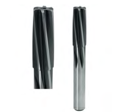
Hand-reamers HSS-E, tolerance H7, straight shank with square end, left hand spiral 7-8°, right hand cutting.
